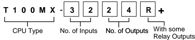
In the above example T100MX-3224+ means that the PLC has 32 ON/OFF type inputs and 24 ON/OFF type outputs. The "R" indicates that some of the outputs are relay type. Models with only transistor-outputs do not carry the "R" label. If you include the 8 channels of analog I/Os, the PLC will have a total of  $32 + 24 + 8 = 64$  I/Os.
