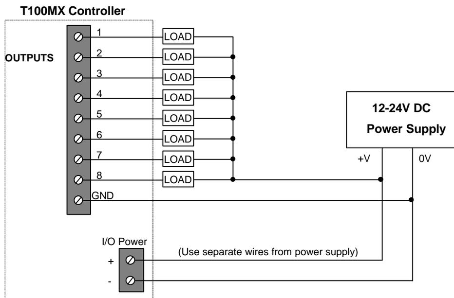
Figure 7 - Transistor Output Interfacing to Load
