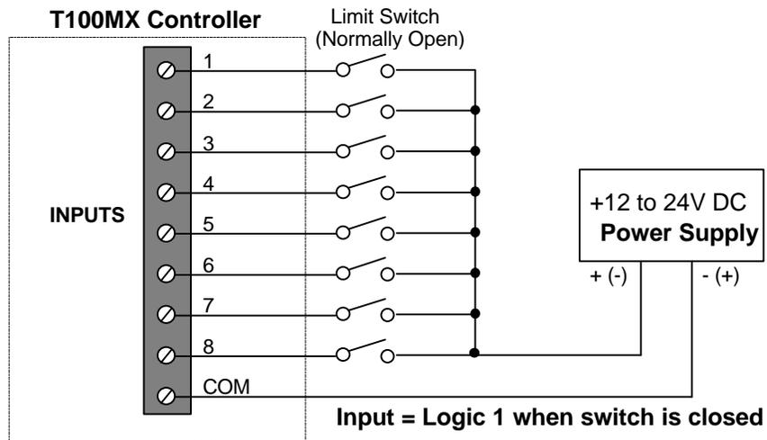
Figure 6 - Input Interfacing to Limit Switches
