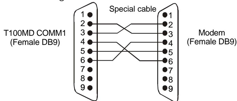
Figure 13 - Connecting COMM1 to a MODEM
