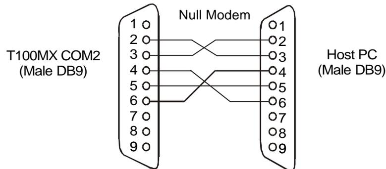
Figure 15 - Connecting COMM2 to a host PC
