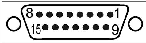
Note that pin #2 and #1 are A/D inputs (AD7 and AD8) after system RESET. You may configure either one or both of them as D/A outputs by executing the "setDAC" command on the respective channel(s). After that they will stay on as D/A outputs until a system RESET has been performed.
