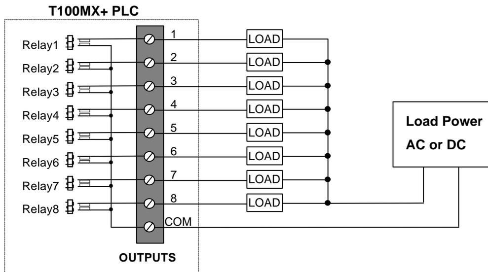
Figure 10 - Relay Output interfacing to load
