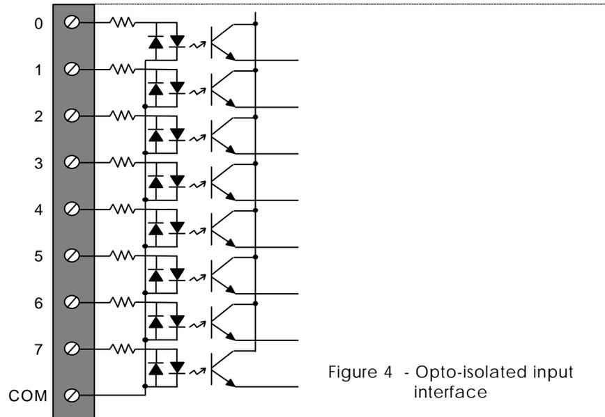
Figure 4 - Opto-isolated input interface
