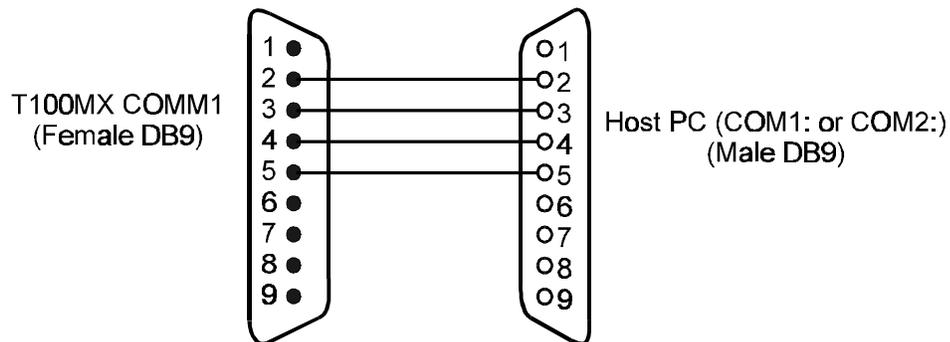
Figure 12 - Connecting COMM1 with PC
