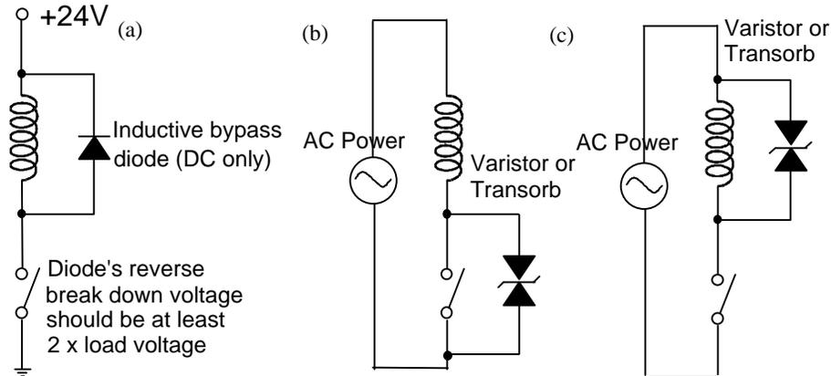
Figure 11 - (a) Inductive snubber circuit - DC load only.
