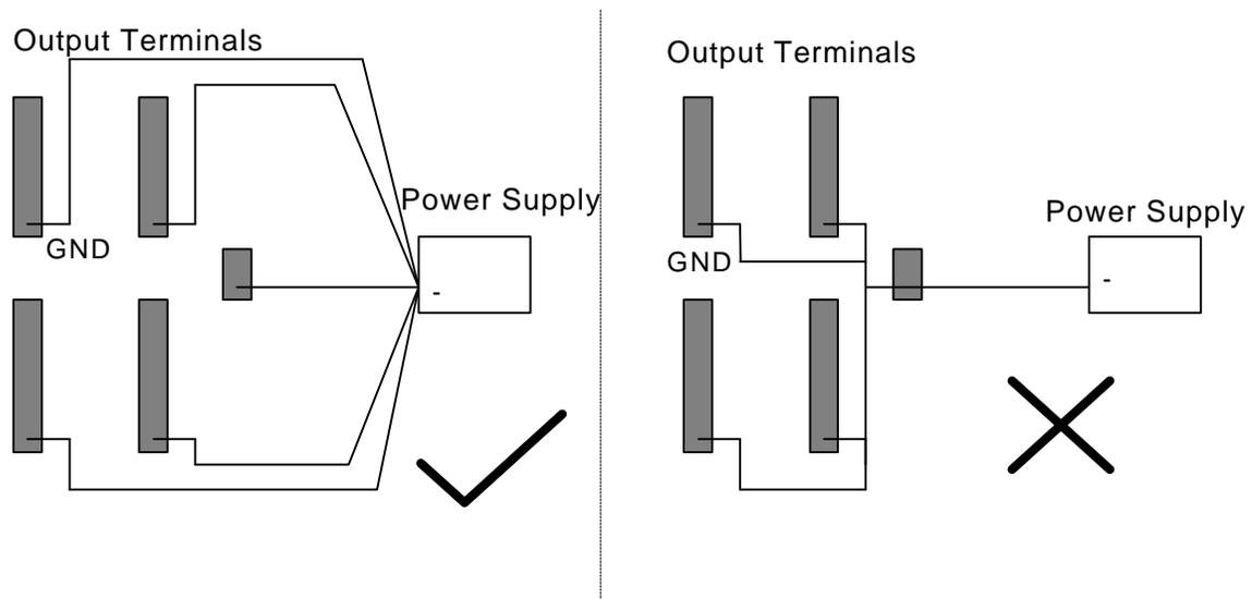
Figure 8 - Preferred Wiring Method of GND terminals
